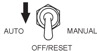
Figure 55. MPEC Control Switch (Off/Reset)
